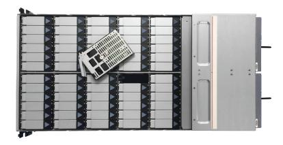
The HGST 4U60 Storage Platform is high density, scalable, and cost effective. With 12Gb/s SAS interface and HDD-SSD hybrid capability, the Platform is designed for data centers that need a dense solution with HA capabilities, while maintaining a low power profile.
